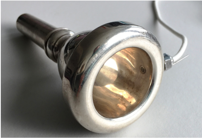
Figure 3: Tuba mouthpiece equipped with pressure transducer.
